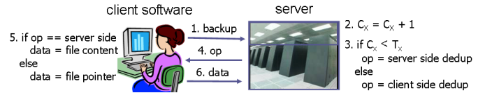
Fig. 1. A Randomized solution. The figure details the operations performed upon the client backup request. For every file the server keeps a random threshold ( T_x ). If the number of existing copies of the document ( C_x ) is at least as high as the threshold, then client side deduplication is performed and the file content are not sent over the network. Otherwise, deduplication is performed only at the server side.
