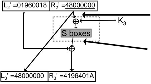
Find which K<sub>3</sub> maps the inputs to an s-box input pair that results in the output pair!
