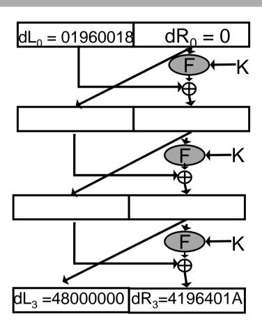
The attacker knows the two plaintext/ciphertext pairs, and therefore also their differences
