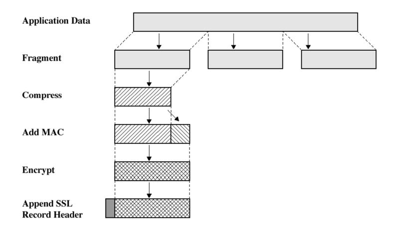
Figure 17.3 SSL Record Protocol Operation
